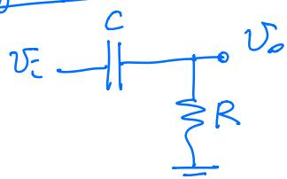
$$\frac{V_o}{V_i} = \frac{R}{\frac{1}{j\omega C} + R} = \frac{j\omega RC}{1 + j\omega RC} = \frac{j\omega}{\underbrace{\frac{1}{RC} + j\omega}_{\omega_L}}$$
